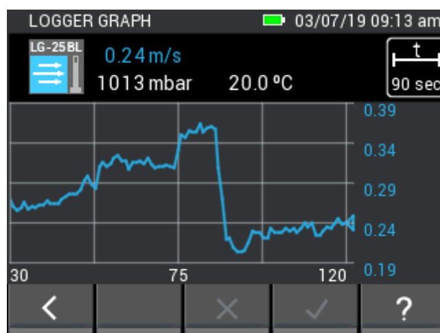
Figure 12-18: Graphical logger measurement with an LG-25 BL sensor
