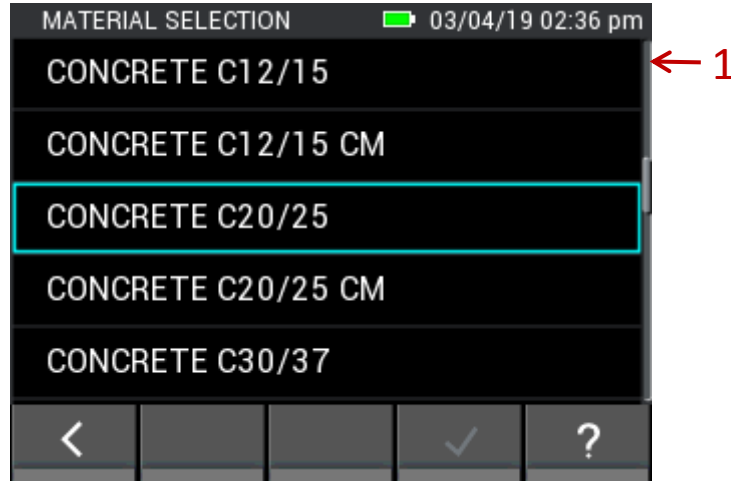
Figure 5-12: Complete building material selection list
