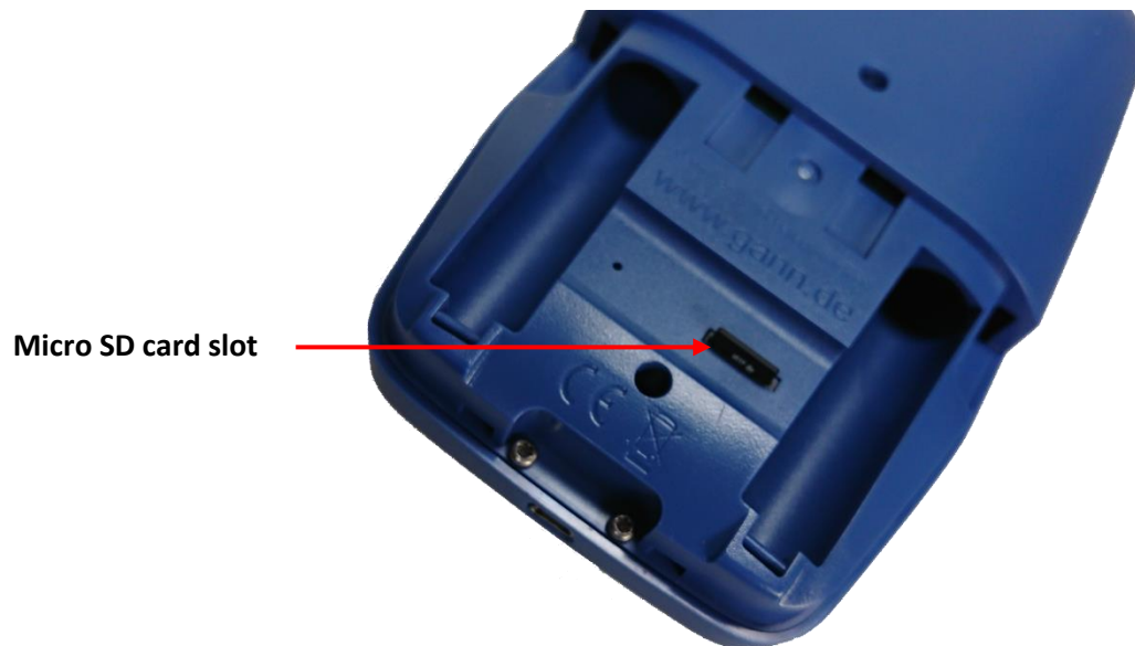
Figure 1-5: Battery compartment with micro SD card slot
